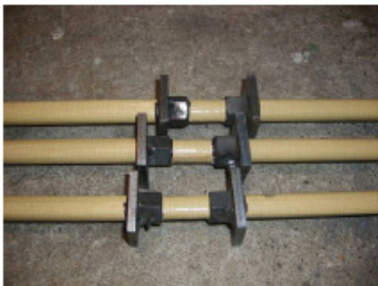
Figure 2.21 Fixing plates used by Shimazaki (2008) to tie the debonded vertical reinforcement together
